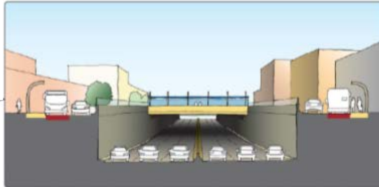
Side-Lane BRT Stations and Overpass - Looking East
